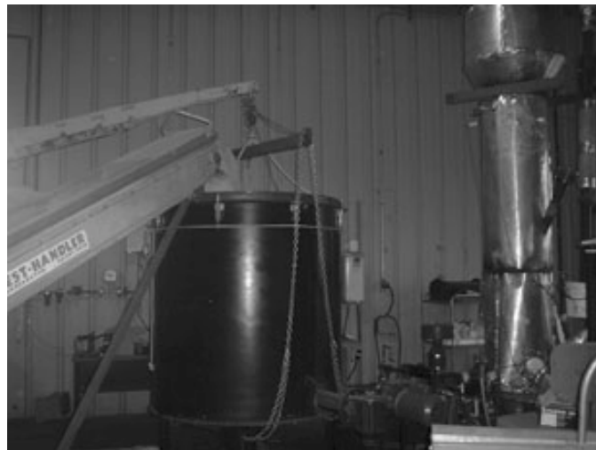
Switchgrass is fed into the hopper then processed through the gasifier.
