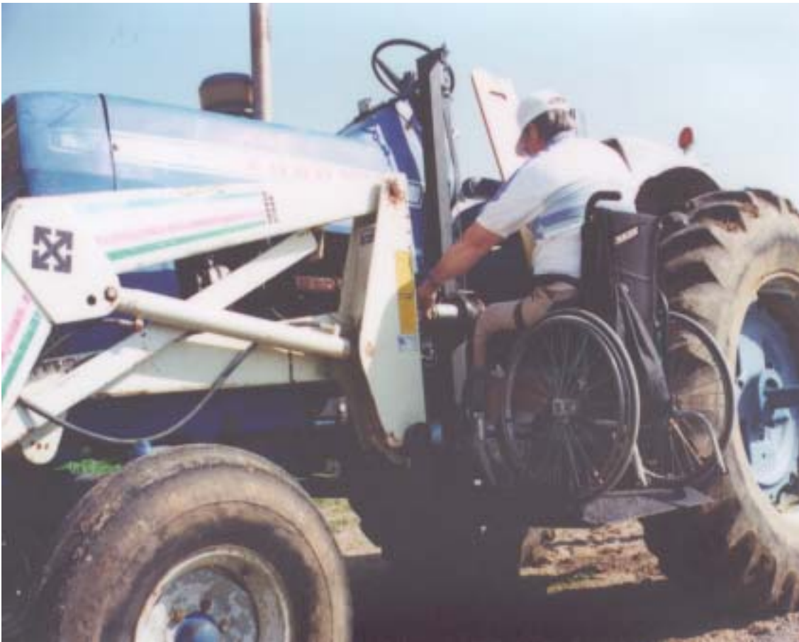
A spinal cord injury left Missouri farmer Lashley Garnett confined to a wheelchair. Today, he uses a wheelchair lift to get onto his tractor. (Photo courtesy of Missouri AgrAbility Project)
