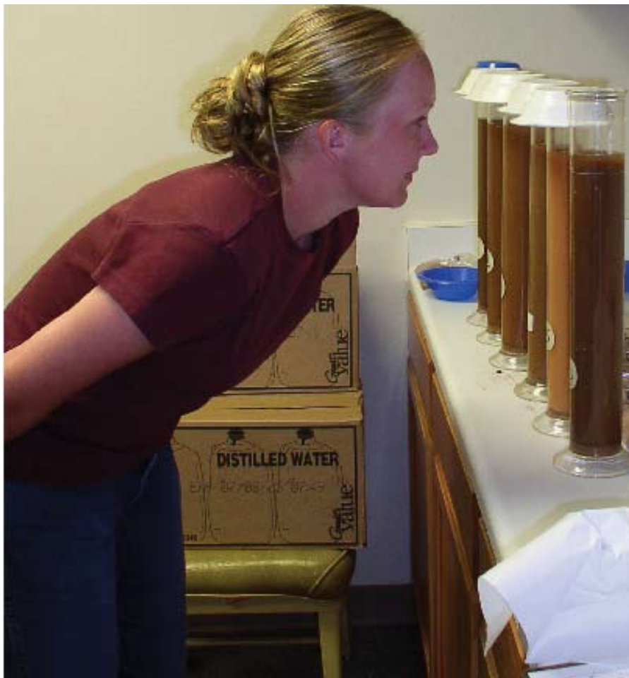
Working with soil does not always have to be dirty. Starr Holtz, a plant and soil sciences graduate student, keeps her hands clean as she runs a particle size analysis on soil samples during her internship with the Natural Resources Conservation Service. (photo courtesy of Starr Holtz)
